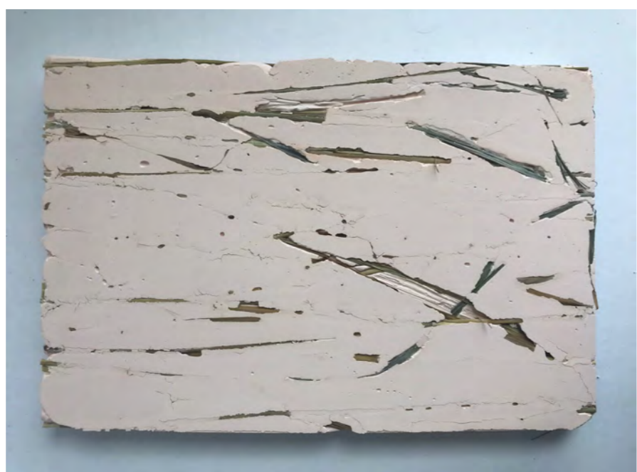
MATERIAL EXPERIMENTS WITH DIFFERENT PATTERNS OF REED WITHIN PINK PIGMENTED CONCRETE
