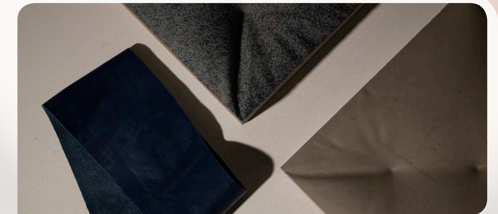
PICTURE 4 - Prototype Flesh (hair) and Grain (smooth) side of leather cast results
