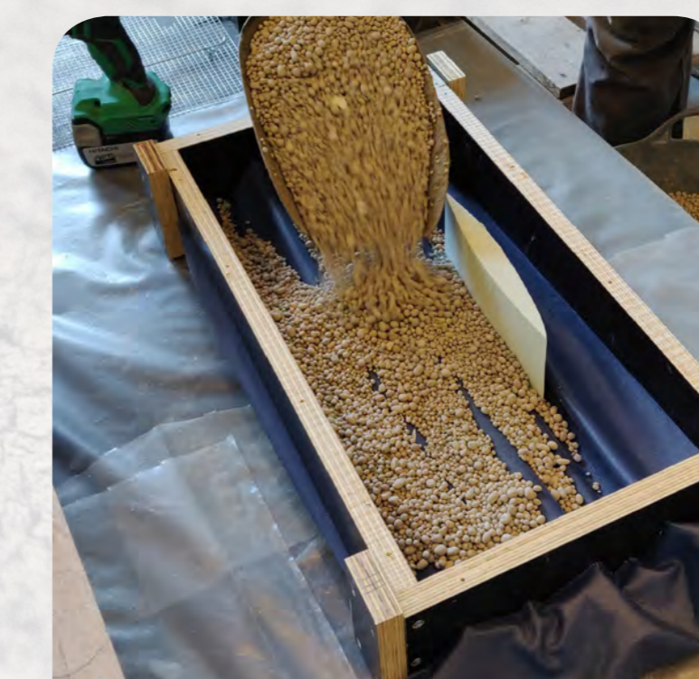
PICTURE 9 - Lower part is reinforced with expanded clay pebbles
